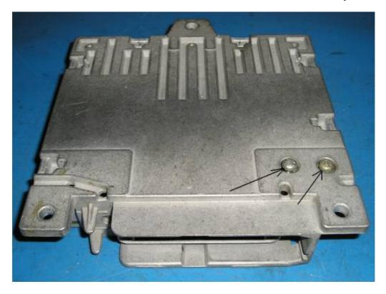
On the base of the unit, unscrew and remove the two heatsink screws indicated in the picture.
