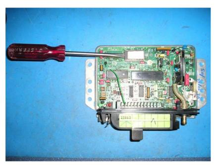
2) Turn the board so the 25way connector is facing you, as below. Carefully insert the new LH EPROM so that the label script can be read.... Make sure all pins are located in their respective sockets and then push the chip fully home. Excess force is not required, if the chip is reluctant to go home, carefully double check the pin locations.
