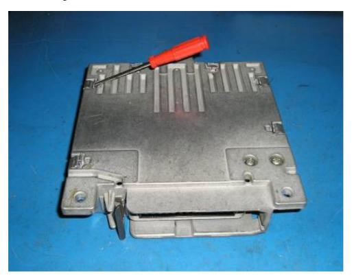
Unscrew and remove the two screws and clip near the 25 way connector. Note that the screw on the right of this picture is a self tapping screw, the other a normal metric threaded screw...
