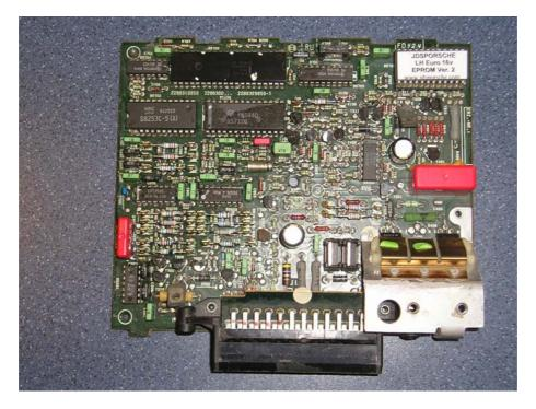
Refit the circuit board to the heatsink plate and clip it into place with the three clips at the rear, then refit the two heatsink screws that were removed in step (5). This is essential for proper heat dissipation in the power semiconductors on the board. If the screws are omitted, damage could result to the devices.
