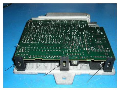
Then by pushing gently on the 25 way connector at the front, and easing the circuit board up at the back, slide the circuit board out of the heatsink frame.
