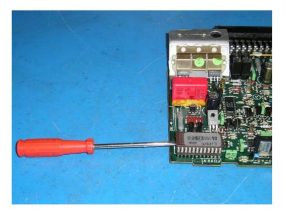
Turn the board so the 25way connector is facing you, as below. Carefully insert the new LH EPRO so that the label script can be read.... Make sure all pins are located in their respective sockets and then push the chip fully home. Excess force is not required; if the chip is reluctant to go home, carefully double check the pin locations.
